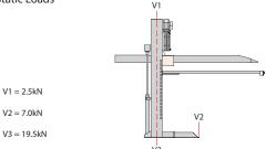
Static load calculations include a vehicle of the maximum weight (2700kg)
